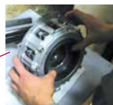
① エンドカバーを手で反転 Turn over the end cover by hand.
