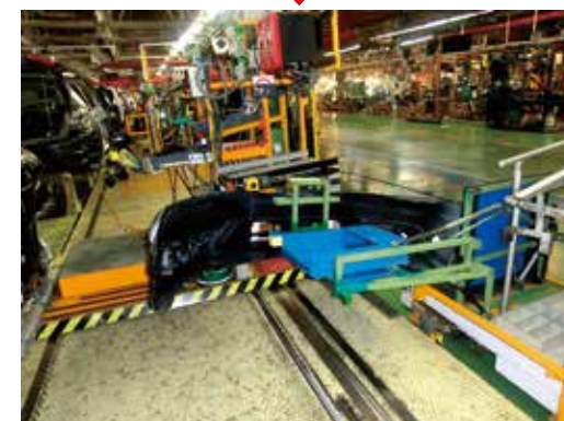
搬送の際は立った状態で運ばれてきたバンパーが作業時には倒れる仕組み。 The bumper, delivered standing up, is lowered when it is worked on.
